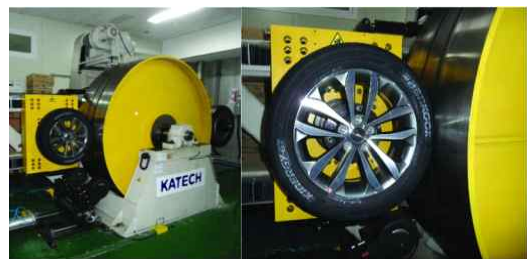
Fig. 3 Photographs of RR measurement system
